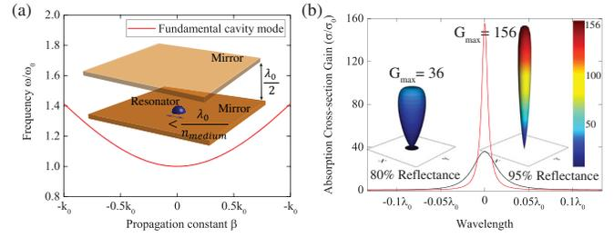
FIG 3 (color online). (a) Schematic of the near-zero phase index structure consisting of two mirrors. The dispersion curve is obtained assuming the mirror has 100% reflection. (b) The spectra of the absorption cross section for mirrors with 80% (black solid line) and 95% (red solid line) reflectance. Insets show the angular response for both cases.
